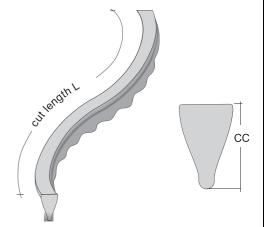
The Aal stable is a surface spacer and is predominantly used in areas such as floor slabs, foundations, etc., with horizontal reinforcement. The contact surface is either smooth or with dimples.
